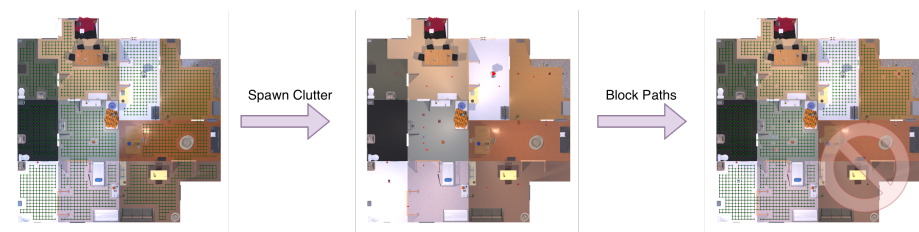
Fig. 1: Example dataset generation process. In this instance, we consider a 10 room floorplan from ProcTHOR-10k. The left image shows the ideal environment without clutter and completely free for optimal navigation throughout the environment. We then generate clutter in the free space using the between-ness centrality of nodes in G_{\text{free}} . The generated obstacle locations are indicated by red circles in the middle image. This causes the blocking of the paths within the accessible rooms, as well as eliminating access to the two rooms on bottom-right of the map, as shown in the right image.
