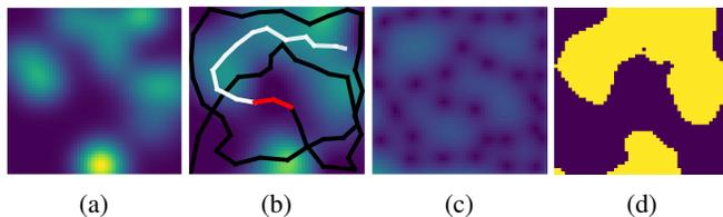
Figure 1: CATnIPP’s *trajectory sampling variant for adaptive IPP*, showing the path executed by the agent so far (black), and the long-horizon trajectory that was just (re-)planned (white), of which the red portion will be executed until the next replanning step. a) True interest map (unknown to the agent), b) Predicted interest map from all measurements so far, c) Associated predicted standard deviation, and d) Predicted high-interest areas.
