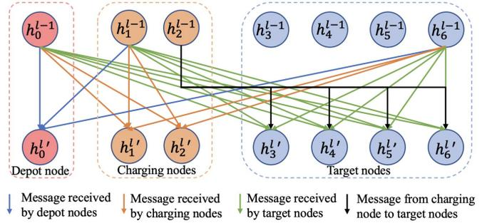
Fig. 3: Illustration of our multi-head heterogeneous attention for an instance with a depot, two charging stations and four target nodes.
