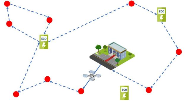
Fig. 1: Example path allowing a UAV to cover all monitoring targets while visiting several stations for recharging along the way.
