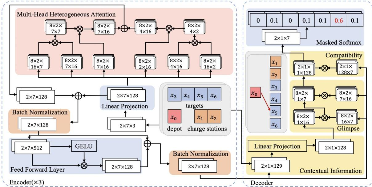
Fig. 2: Illustration of our neural network for two instances with a depot, two charging stations, and four target nodes. The neural network consists of an encoder with three attention layers and a decoder with a multi-head attention layer and a single head attention layer.
