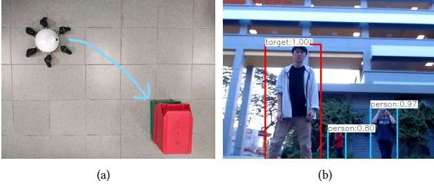
Figure 8: (a) Hexa robot walk towards the red box on the left front with its trajectory (blue line). (b) Daisy perspective when the robot is tracking people (the bounding box in red is target, the bounding box in blue is other objects in frame).
